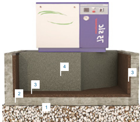
1. Riprap 2. Reinforced concrete slab 3. Expanded Cork Board - ICB High Density 4. Reinforced concrete affixation
